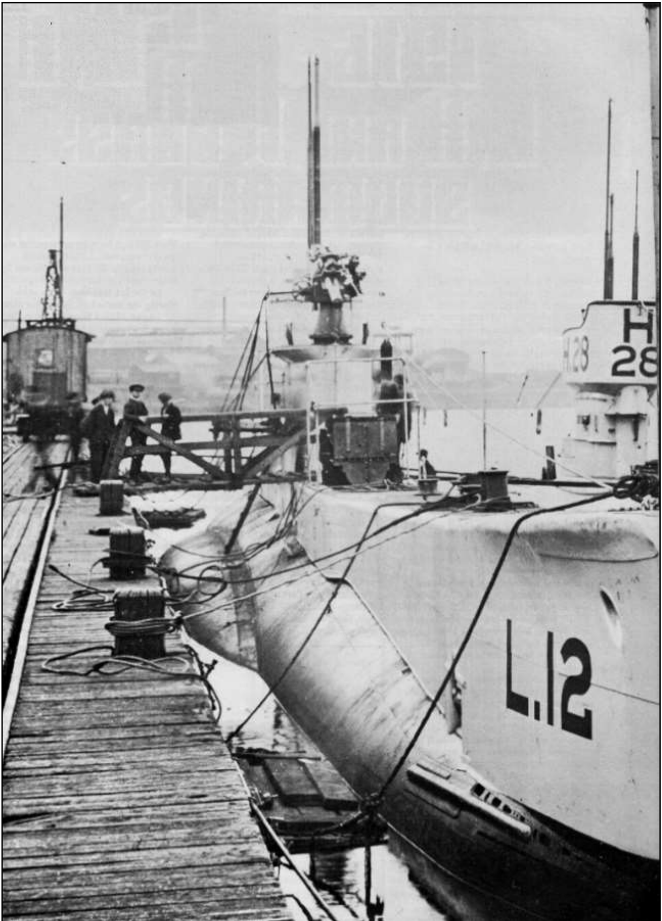
L12 and H28 fitting out in Devonshire Dock in May/June 1918. Note L12s saddle tank construction and the 4-inch gun mounting.
