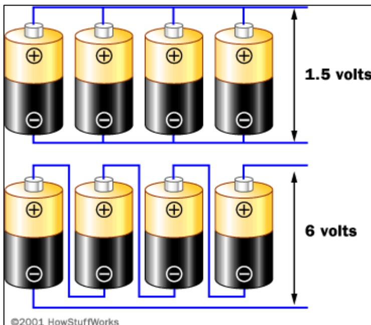
In almost any device that uses batteries, you do not use just one cell at a time. You normally group them together serially to form higher voltages, or in parallel to form higher currents. In a serial arrangement, the voltages add up. In a parallel arrangement, the currents add up. The following diagram shows these two arrangements:
