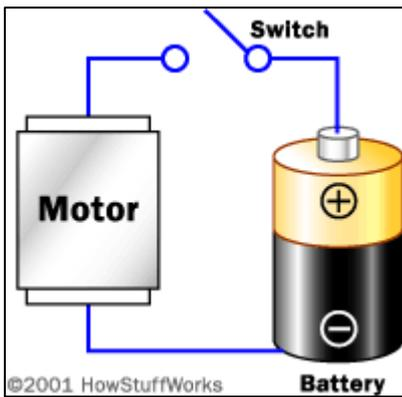
If you look at any battery, you'll notice that it has two terminals. One terminal is marked (+), or positive, while the other is marked (-), or negative. In an AA, C or D cell (normal flashlight batteries), the ends of the battery are the terminals. In a large car battery, there are two heavy lead posts that act as the terminals.
