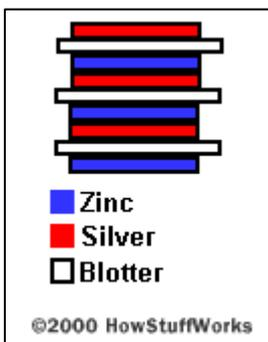
The first battery was created by Alessandro Volta in 1800. To create his battery, he made a stack by alternating layers of zinc, blotting paper soaked in salt water, and silver, like this:
