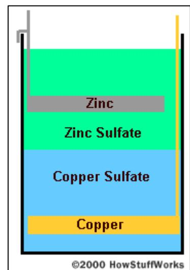
There is less heat. You can power a light bulb or similar load using the electrons flowing through the wire, and you can measure a voltage and current in the wire. Some of the heat energy is turned into electron motion.
