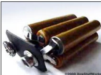
If you arrange four of these 1.25-volt, 500 milliamp-hour batteries in a serial arrangement, you get 5 volts ( $1.25 \times 4$ ) at 500 milliamp-hours. If you arrange them in parallel, you get 1.25 volts at 2,000 ( $500 \times 4$ ) milliamp-hours. Have you ever looked inside a normal 9-volt battery? It contains six, very small batteries
