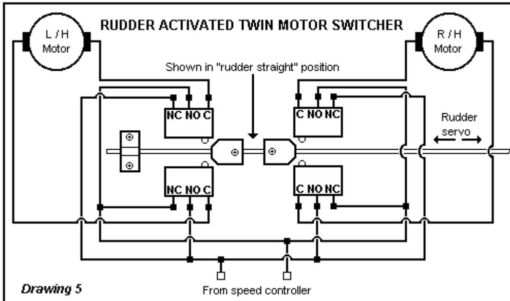
A guide to switching twin-motored boats from the rudder by micro switches and without the added expense of mixers.
