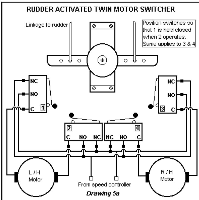
find that by using either roller or lever micro switches it makes it a lot easier to position them correctly.
