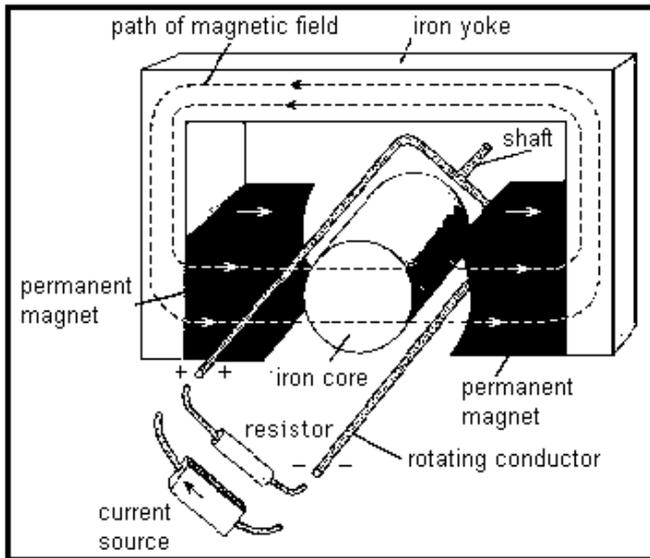
In an elementary form of a DC motor, a stationary magnetic field is produced across the rotor by poles on the stator. These poles may be encircled by field coils carrying direct current, or they may contain permanent magnets. The rotor or armature consists of an iron core with a coil accommodated in slots. The ends of the coil are connected to the bars of a commutator switch mounted on the rotor shaft. Stationary graphite brushes lead to external terminals.
