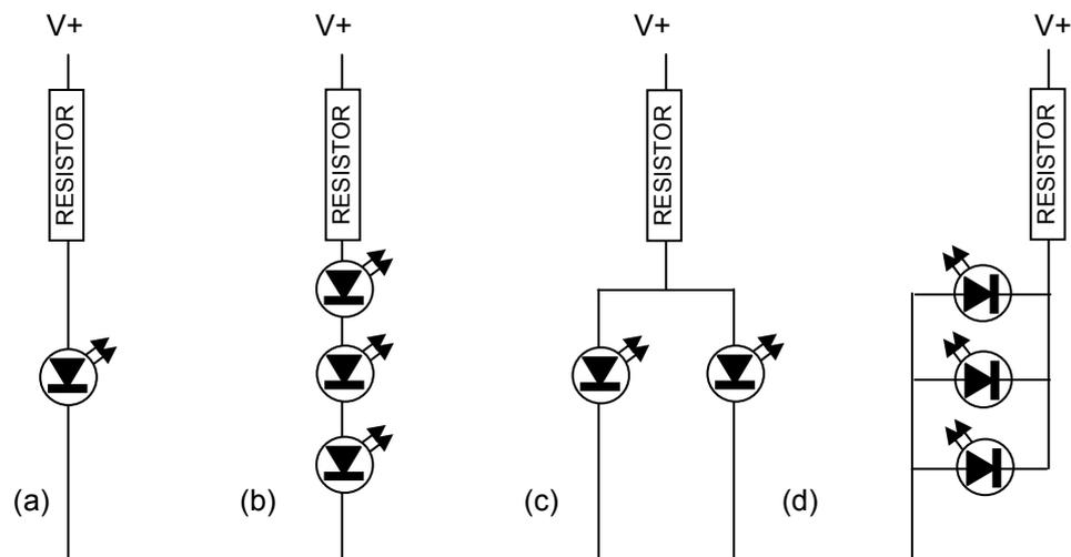
It should also be noted that LEDs are polarised, that means that they will only work when the negative supply is connected to the Cathode.
