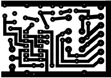
**Fig 12** Printed Board Master (actual size 42 x 60mm)
