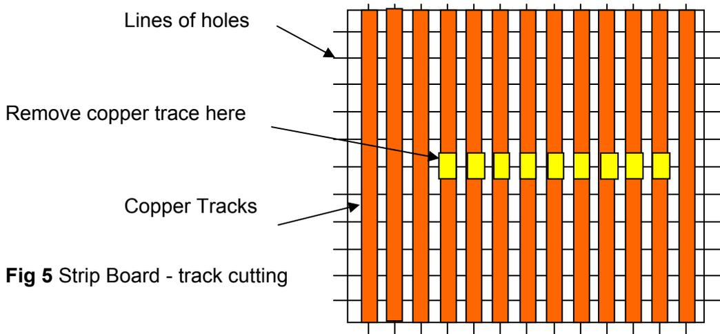
**Fig 5** Strip Board - track cutting
