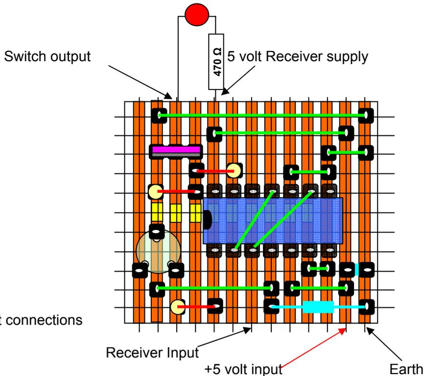
Fig 8 Test connections
