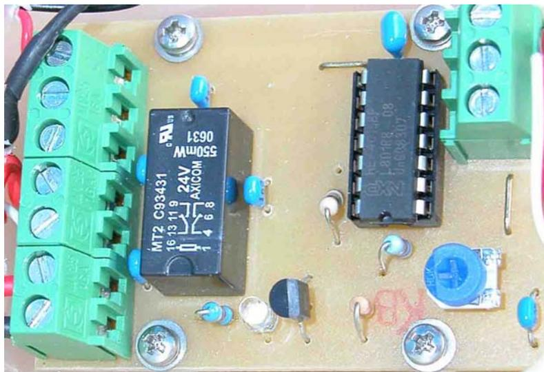
**Fig 13** Completed Electronic Switch with Relay Output
