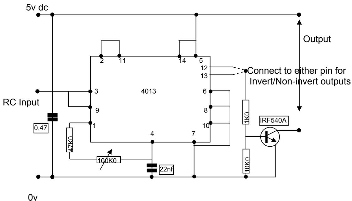
**Fig 1** Schematic Diagram of Single RC Switch
