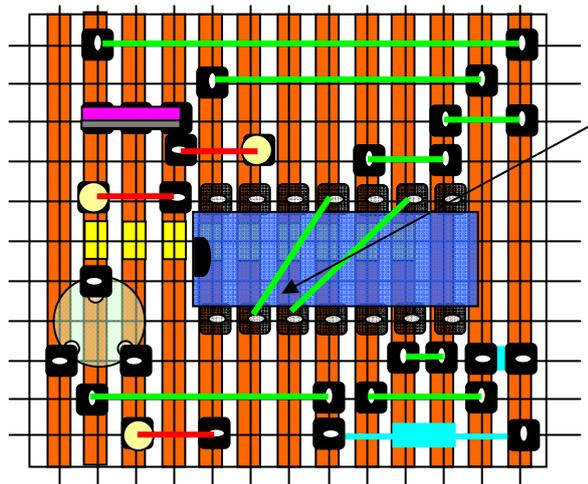
Add these two links across the IC pins on track side of the board - insulate from the copper tracks.
