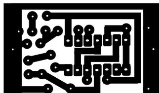
**Fig 4** PCB Master (Scale 1:1) for the list of components see appendix A.
