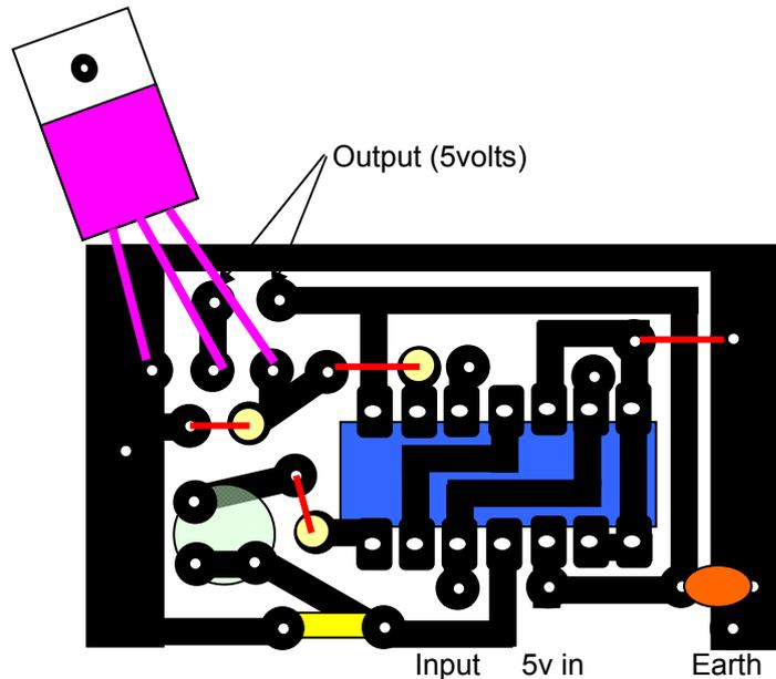
**Fig 3** Switch PCB Component Layout (Scale 2:1) PCB actual size 42 x 24mm see Fig 4.
