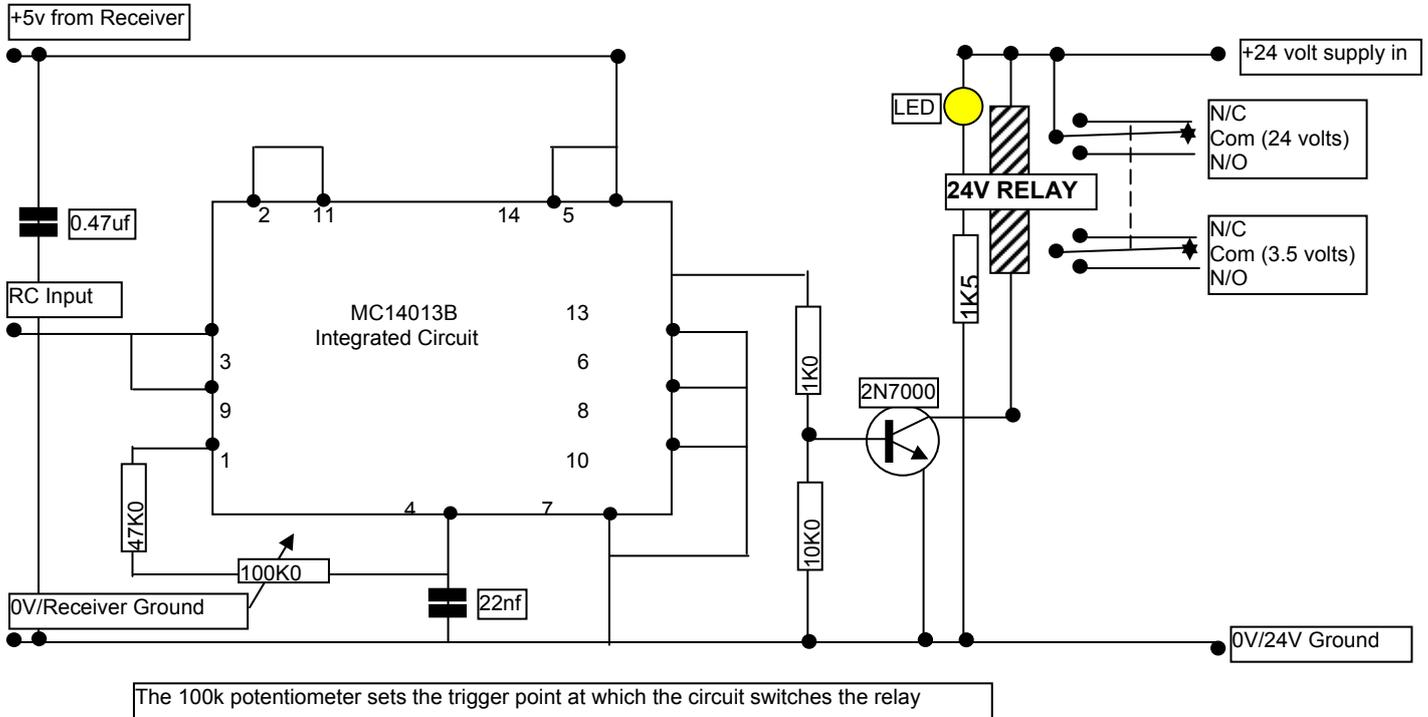
**Fig 10** Circuit diagram of the electronic switch with relay output.
